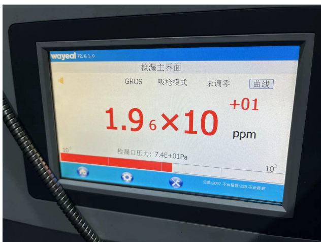
阀体密封最大泄漏量 Max.leakage from body seals
