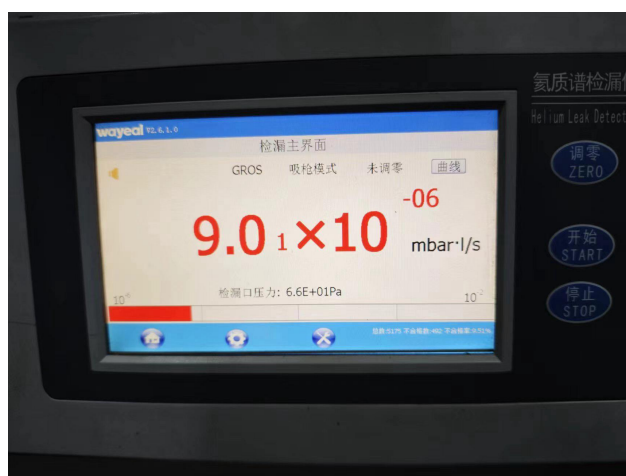
阀杆密封最大泄漏量 Max.leakage from stem seals
