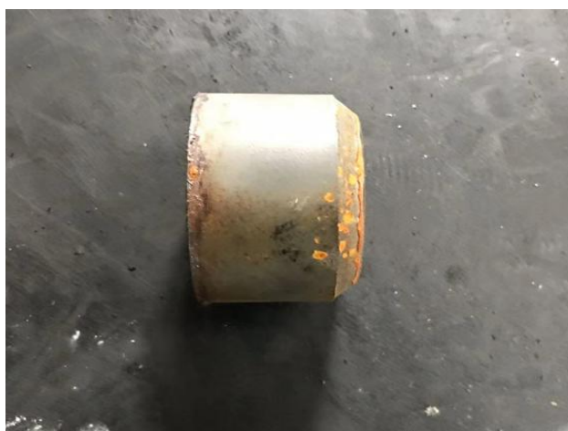
拆卸后衬套 Bushing after removal
