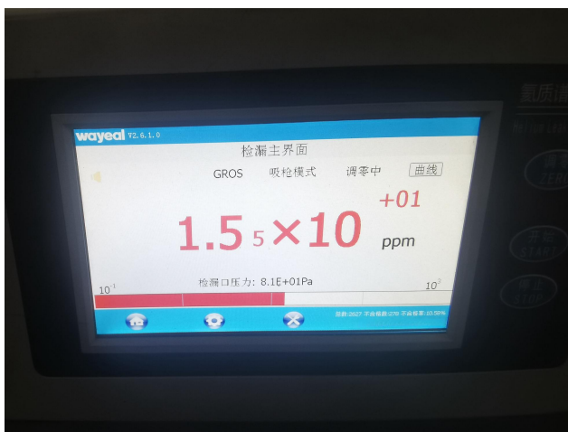
阀体密封最大泄漏量 Max.leakage from body seals
